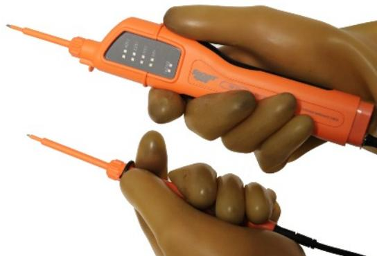
Check the VIP ESI's operation before and after use on the SP400WPD proving unit (SOC/SP400WPD)
