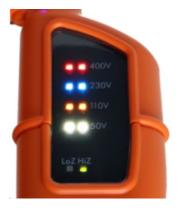
If this indication is given, further checks can be carried out using a Fluke 116 DMM. On Volts AC setting a voltage will be indicated, on LoZ setting the voltage will be dissipated.
