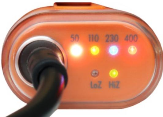
To measure voltage, touch the prods onto the circuit to be measured. Ensure there is a firm and clean contact.
