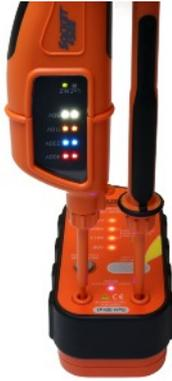
Note the VIP ESI indicates on LEDs both on the main body and the end cap of the tester to allow clear indication in a link box or other confined spaces.
