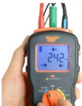
GOOD socket test and mains voltage
