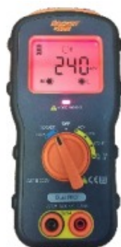
Fault condition missing earth
