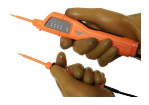
Check the VIP ESI's operation before and after use on the SP400 proving unit (SOC/SP400)
