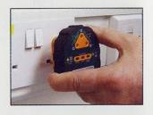
2 Switch on. When first powered up the LEDs in the orange triangle flash green then red once as it performs a self test. This is immediately followed by a
