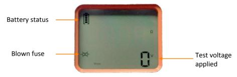
\*LCD is shown indicating a blown fuse.
